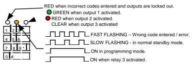
To activate your gates or door via keypad, simply enter the 4 digit code which has been programmed by your installer.
